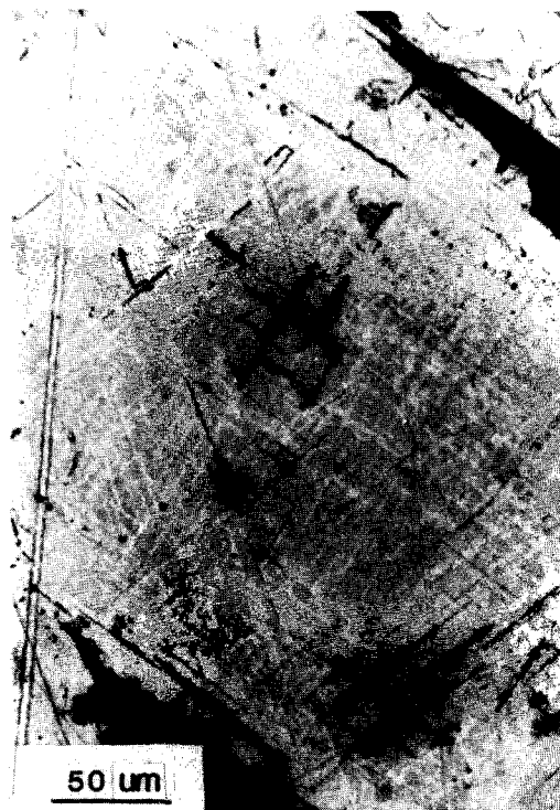
FIG. 2. Light micrograph of a polished section of a prerduced granule showing the extent of the reduction reaction. The parent magnetite grains contain a high density of crystallographically oriented channels.
