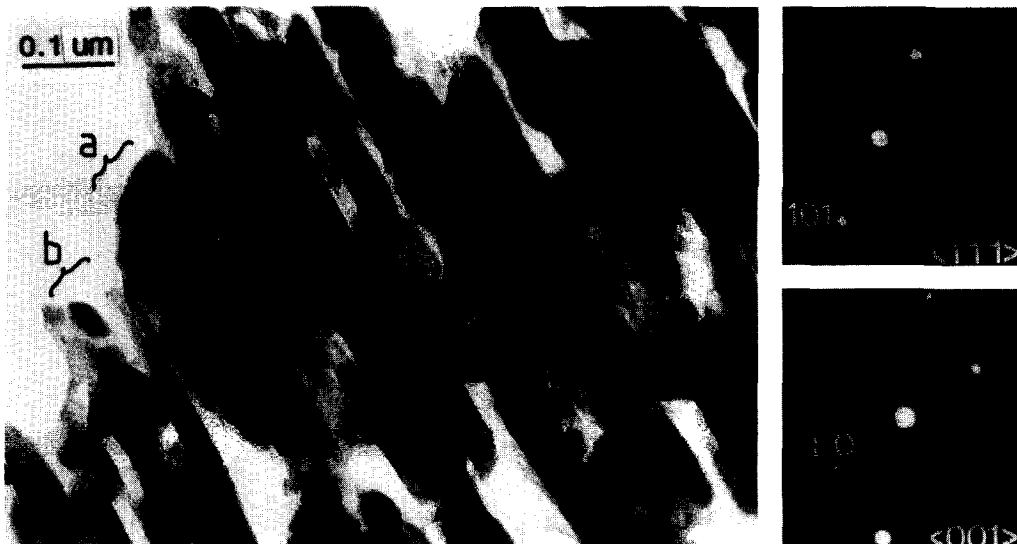
FIG. 11. Bright field transmission electron micrograph of prereduced material showing long crystals, which interpenetrated more blocky crystals of \alpha -iron. Also shown are the microbeam diffraction patterns from adjacent long crystal regions; region a exhibited a \langle 100 \rangle zone axis and region b , a \langle 111 \rangle zone axis.
