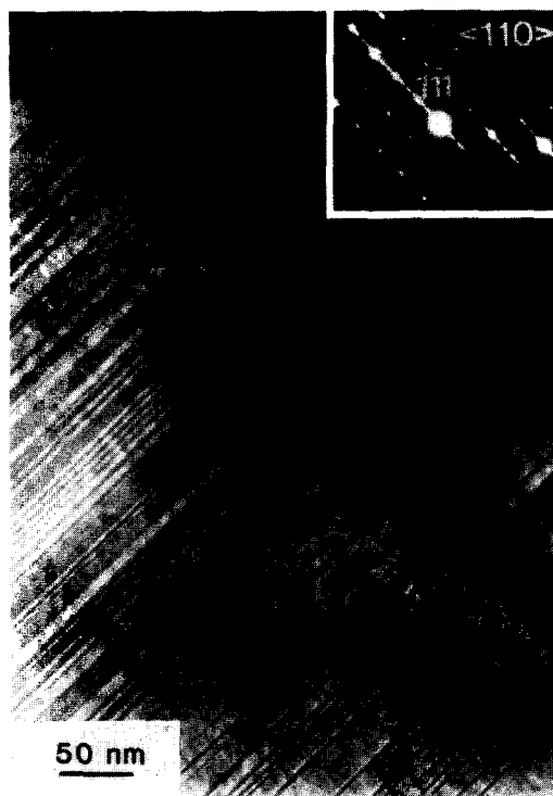
FIG. 1. Transmission electron micrograph of a finely faulted region of magnetite and the corresponding diffraction pattern (inset) showing extensive faulting on {111} planes.
